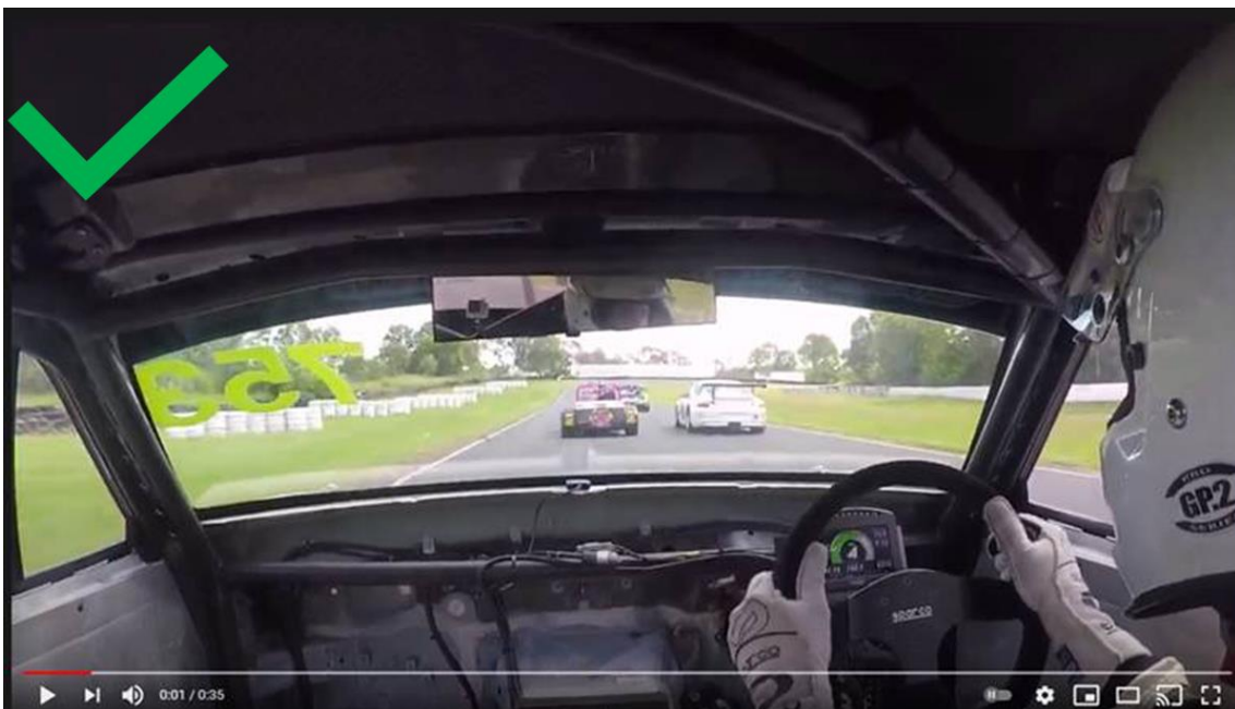
Figure 2 Example of acceptable camera position - A-pillars
